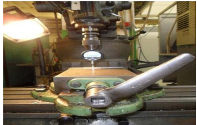
Figure 5. Work piece measurement with digital dial gauge.
