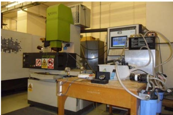
Figure 1. Electrochemical machining system rig.
